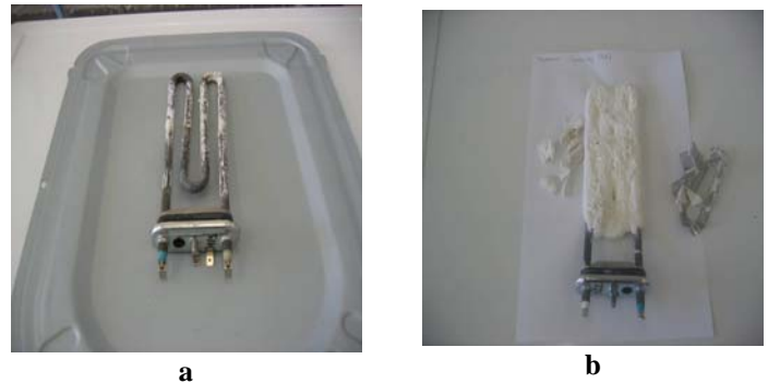
Fig. 7 washing machine heaters after 300 cycles of washing without washing powders (a – at 60°C, b – at 95°C)
